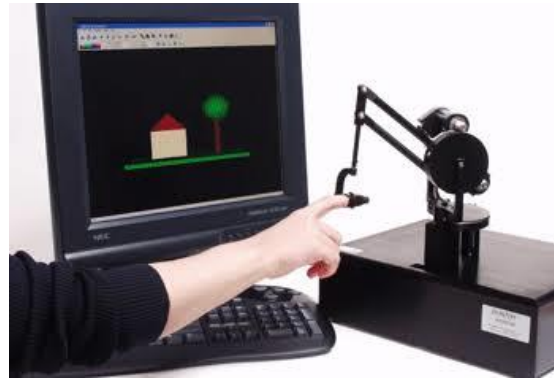
Fig: 4 Phantom (Haptic Device)
