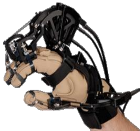
Fig 4: Cyber glove (Haptic Device)
